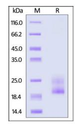
Human TRBC1, His Tag on SDS-PAGE under reducing (R) condition. The gel was stained overnight with Coomassie Blue. The purity of the protein is greater than 90%.
