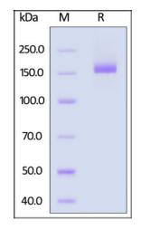
SARS-CoV-2 Spike Trimer, His Tag (BA.3/Omicron) on SDS-PAGE under reducing (R) condition. The gel was stained overnight with Coomassie Blue. The purity of the protein is greater than 95%.
