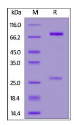
Anti-SARS-CoV-2 Spike RBD Neutralizing Antibody, Chimeric mAb, Human IgM (AM122) on SDS-PAGE under reducing (R) condition. The gel was stained overnight with Coomassie Blue. The purity of the protein is greater than 95%.
