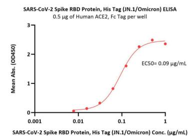
Immobilized Human ACE2, Fc Tag (Cat. No. AC2-H5257) at 5  $\mu$ g/mL (100  $\mu$ L/well) can bind SARS-CoV-2 Spike RBD Protein, His Tag (JN.1/Omicron) (Cat. No. SPD-C5249) with a linear range of 0.008-0.25  $\mu$ g/mL (Routinely tested).
