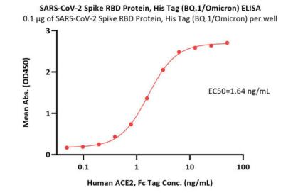
Immobilized SARS-CoV-2 Spike RBD Protein, His Tag (BQ.1/Omicron) (Cat. No. SPD-C5243) at 1  $\mu$ g/mL (100  $\mu$ L/well) can bind Human ACE2, Fc Tag (Cat. No. AC2-H5257) with a linear range of 0.1-3 ng/mL (Routinely tested).
