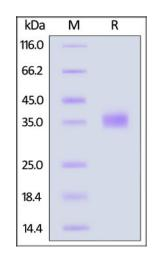
SARS-CoV-2 Spike RBD, His Tag (BQ.1.1/Omicron) on SDS-PAGE under reducing (R) condition. The gel was stained overnight with Coomassie Blue. The purity of the protein is greater than 95%.
