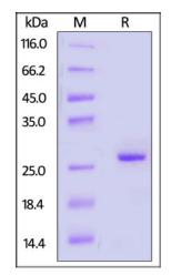
RNase III ( $2U/\mu l$ ) on SDS-PAGE under reducing (R) condition. The gel was stained with Coomassie Blue. The purity of the protein is greater than 90%.
