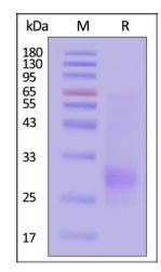
Biotinylated Mouse PVRIG Protein, His, Avitag on SDS-PAGE under reducing (R) condition. The gel was stained with Coomassie Blue. The purity of the protein is greater than 90% (With <u>Star Ribbon Pre-stained Protein Marker</u>).
