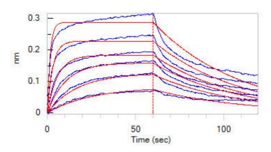
Loaded Canine PD-1, His Tag (Cat. No. PD1-C52H9) on HIS1K Biosensor, can bind Canine PD-L1, Fc Tag (Cat. No. PD1-C52H3) with an affinity constant of 85 nM as determined in BLI assay (ForteBio Octet Red96e) (Routinely tested).
