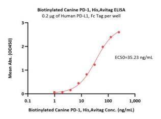
Immobilized Human PD-L1, Fc Tag (Cat. No. PD1-H5258) at 2  $\mu$ g/mL (100  $\mu$ L/well) can bind Biotinylated Canine PD-1, His,Avitag (Cat. No. PD1-C52E5) with a linear range of 1-63 ng/mL (QC tested).
