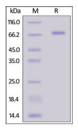
Biotinylated Mouse CD200, Fc, Avitag on SDS-PAGE under reducing (R) condition. The gel was stained overnight with Coomassie Blue. The purity of the protein is greater than 95%.
