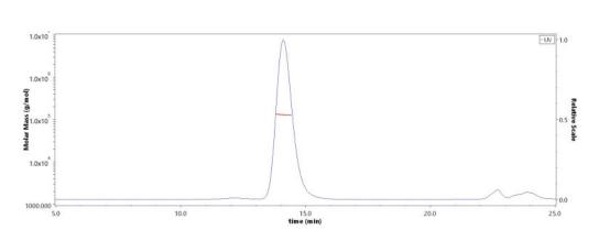
The purity of Biotinylated Mouse CD200, Fc, Avitag (Cat. No. OX2-M82F3) is more than 90% and the molecular weight of this protein is around 125-135 kDa verified by SEC-MALS.
