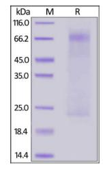
MERS Nucleocapsid protein, His Tag on SDS-PAGE under reducing (R) condition. The gel was stained overnight with Coomassie Blue. The purity of the protein is greater than 90%.
