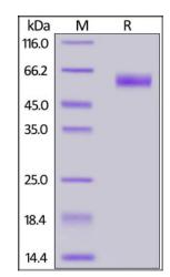
SARS-CoV-2 Nucleocapsid protein, His Tag on SDS-PAGE under reducing (R) condition. The gel was stained with Coomassie Blue. The purity of the protein is greater than 95%.
