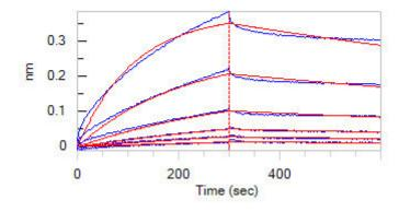
Loaded Human NOTCH2, Fc Tag (Cat. No. NO2-H5255) on Protein A Biosensor, can bind Human DLL4, His Tag (Cat. No. DL4-H5227) with an affinity constant of 77.6 nM as determined in BLI assay (ForteBio Octet Red96e) (Routinely tested).
