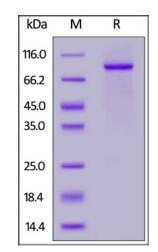
Human NOTCH2, Fc Tag on SDS-PAGE under reducing (R) condition. The gel was stained with Coomassie Blue. The purity of the protein is greater than 95%.
