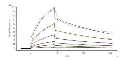
Influenza B [PHUKET/3073/2013] Neuraminidase (NA) Protein, His Tag (Cat. No. NEE-V5246) immobilized on CM5 Chip can bind N-Acetylneuraminic Acid (NANA,Neu5Ac) with an affinity constant of 1.11 mM as determined in a SPR assay (Biacore 8K) (QC tested).
