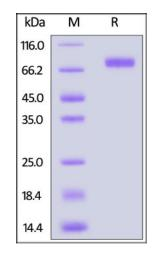
Rat NKG2A&CD94 Protein, Mouse IgG2a Fc Tag on SDS-PAGE under reducing (R) condition. The gel was stained overnight with Coomassie Blue. The purity of the protein is greater than 95%.
