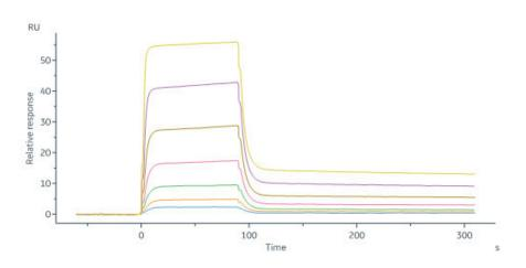
Human MCAM, His Tag (Cat. No. CD6-H5229) captured on CM5 chip via anti-His antibody can bind Human Laminin 411 Protein (Cat. No. LAT-H5263) with an affinity constant of 27.9 nM as determined in a SPR assay (Biacore 8K) (Routinely tested).
