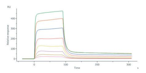
Human MCAM, His Tag (Cat. No. CD6-H5229) immobilized on CM5 Chip can bind Human Laminin 411 Protein (Cat. No. LAT-H5263) with an affinity constant of  $0.115~\mu M$  as determined in a SPR assay (Biacore 8K) (Routinely tested).
