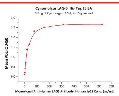
Immobilized Cynomolgus LAG-3, His Tag (Cat. No. <u>LA3-C82H3</u>) at 2  $\mu$ g/mL (100  $\mu$ L/well) can bind Monoclonal Anti-Human LAG3 Antibody, Human IgG1 with a linear range of 1-78 ng/mL (QC tested).
