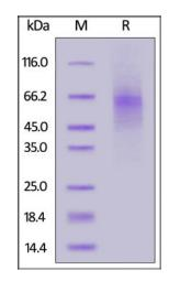
Cynomolgus LAG-3, His Tag on SDS-PAGE under reducing (R) condition. The gel was stained overnight with Coomassie Blue. The purity of the protein is greater than 90%.
