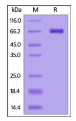
Human KIR2DL3, Fc Tag on SDS-PAGE under reducing (R) condition. The gel was stained overnight with Coomassie Blue. The purity of the protein is greater than 95%.
