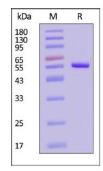
Canine IRAK4 Protein, His Tag on SDS-PAGE under reducing (R) condition. The gel was stained with Coomassie Blue. The purity of the protein is greater than 95% (With <u>Star Ribbon Pre-stained Protein Marker</u>).
