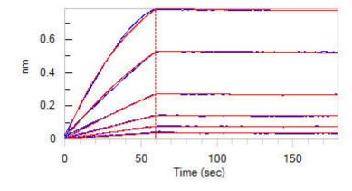
Loaded Biotinylated Human IL-10 R alpha, Fc,Avitag (Cat. No. ILR-H82F6) on SA Biosensor, can bind Human IL-10, His Tag (Cat. No. IL0-H4248) with an affinity constant of 0.72 nM as determined in BLI assay (ForteBio Octet Red96e) (Routinely tested).
