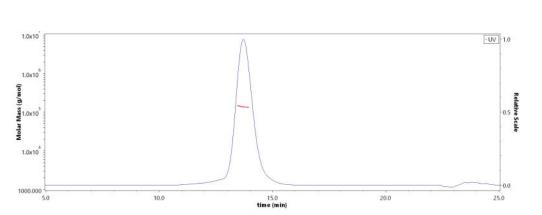
The purity of Biotinylated Human IL-10 R alpha, Fc, Avitag (Cat. No. ILR-H82F6) is more than 90% and the molecular weight of this protein is around 124-152 kDa verified by SEC-MALS.
