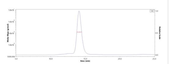
The purity of Mouse IL-2RB&IL-2RG Heterodimer Protein, His Tag&Twin-Strep Tag (Cat. No. ILG-M5283) is more than 85% and the molecular weight of this protein is around 110-125 kDa verified by SEC-MALS.
