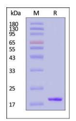
Mouse IL-1 beta, His Tag on SDS-PAGE under reducing (R) condition. The gel was stained with Coomassie Blue. The purity of the protein is greater than 95% (With <u>Star Ribbon Pre-stained Protein Marker</u>).
