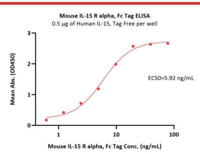
Immobilized Human IL-15, premium grade (Cat. No. IL5-H4117) at 5  $\mu$ g/mL (100  $\mu$ L/well) can bind Mouse IL-15 R alpha, Fc Tag (Cat. No. ILA-M5253) with a linear range of 0.6-10 ng/mL (QC tested).
