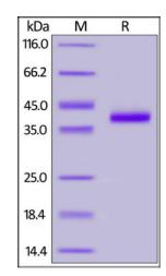
Human IL-8, Fc Tag on SDS-PAGE under reducing (R) condition. The gel was stained with Coomassie Blue. The purity of the protein is greater than 95%.
