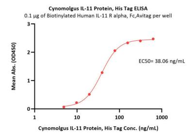
Immobilized Biotinylated Human IL-11 R alpha, Fc,Avitag (Cat. No. ILR-H82F5) at 1  $\mu$ g/mL (100  $\mu$ L/well) on streptavidin (Cat. No. STN-N5116) precoated (0.5  $\mu$ g/well) plate can bind Cynomolgus IL-11 Protein, His Tag (Cat. No. IL1-C5243) with a linear range of 5-156 ng/mL (QC tested).
