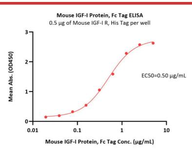
Immobilized Mouse IGF-I R, His Tag (Cat. No. IGR-M5223) at 5  $\mu$ g/mL (100  $\mu$ L/well) can bind Mouse IGF-I Protein, Fc Tag (Cat. No. IG1-M5253) with a linear range of 0.02-1.25  $\mu$ g/mL (QC tested).
