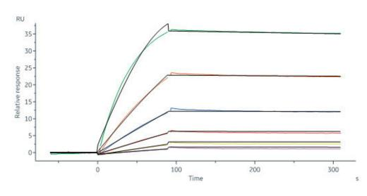
Monoclonal Anti-IFNγ antibody, Human IgG1 (13E6H6) (Cat. No. IFN-M414) captured on CM5 chip via Anti-human IgG Fc antibodies surface can bind Human IFN-gamma, premium grade (Cat. No. IFG-H4211) with an affinity constant of 0.11 nM as determined in a SPR assay (Biacore 8K) (Routinely tested).
