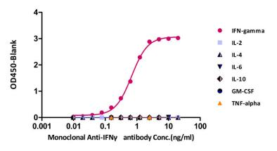
Immobilized Human IFN-gamma, premium grade (Cat. No. IFG-H4211) can bind Monoclonal Anti-IFN $\gamma$  antibody, Human IgG1 (13E6H6) (Cat. No. IFN-M414) with a linear range of 0.07-0.63 ng/mL (QC tested). No cross-reactivity is detected with other human cytokines, including IL-2, IL-4, IL-6, IL-10, GM-CSF and TNF-alpha.
