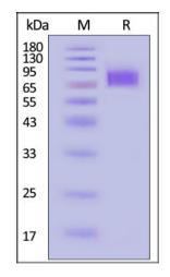
Cynomolgus IFN-alpha/beta R1 Protein, His Tag on SDS-PAGE under reducing (R) condition. The gel was stained with Coomassie Blue. The purity of the protein is greater than 90% (With <u>Star Ribbon Pre-stained Protein Marker</u>).
