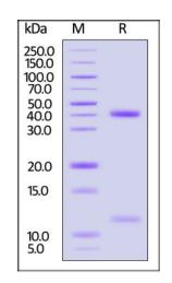
Biotinylated Human HLA-A\*11:01&B2M&KRAS (VVGAGGVGK) Complex Protein on SDS-PAGE under reducing (R) condition. The gel was stained with Coomassie Blue. The purity of the protein is greater than 90%.
