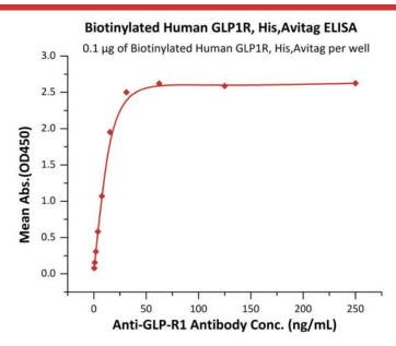
Immobilized Biotinylated Human GLP1R Protein, His,Avitag (Cat. No. GLR-H82E3) at 1  $\mu$ g/mL (100  $\mu$ L/well) on streptavidin (Cat. No. STN-N5116) precoated (0.5  $\mu$ g/well) plate can bind Anti-GLP-R1 Antibody with a linear range of 0.5-31 ng/mL (QC tested).
