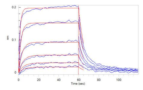
Loaded Biotinylated Human GLP1R, His,Avitag (Cat. No. GLR-H82E3) on NTA Biosensor, can bind GLP-1 (7-37) with an affinity constant of 1.40  $\mu$ M as determined in BLI assay (ForteBio Octet Red96e) (Routinely tested).
