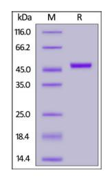
Human GAS6, His Tag on SDS-PAGE under reducing (R) condition. The gel was stained with Coomassie Blue. The purity of the protein is greater than 95%.
