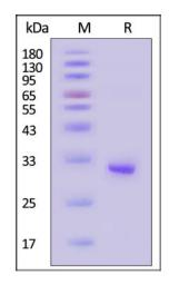
Human FOLR4, His Tag on SDS-PAGE under reducing (R) condition. The gel was stained with Coomassie Blue. The purity of the protein is greater than 95% (With <u>Star Ribbon Pre-stained Protein Marker</u>).
