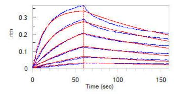
Loaded Biotinylated Human FGL1, Avitag,Fc Tag (Cat. No. FG1-H82F4) on SA Biosensor, can bind Human LAG-3, Fc Tag (Cat. No. LA3-H5255) with an affinity constant of 4.12 nM as determined in BLI assay (ForteBio Octet Red96e) (Routinely tested).
