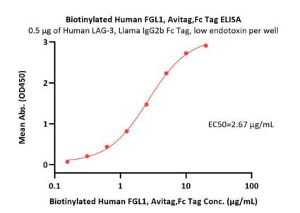
Immobilized Human LAG-3, Llama IgG2b Fc Tag, low endotoxin (Cat. No. LA3-H525c) at 5  $\mu$ g/mL (100  $\mu$ L/well) can bind Biotinylated Human FGL1, Avitag,Fc Tag (Cat. No. FG1-H82F4) with a linear range of 0.156-5  $\mu$ g/mL (QC tested).
