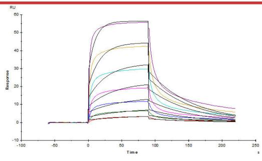
Rhesus macaque CD16, His Tag (Cat. No. FC6-R52H6) captured on CM5 Chip via anti-His antibody can bind Rituximab with an affinity constant of 0.232  $\mu$ M as determined in SPR assay (Biacore T200) (QC tested).
