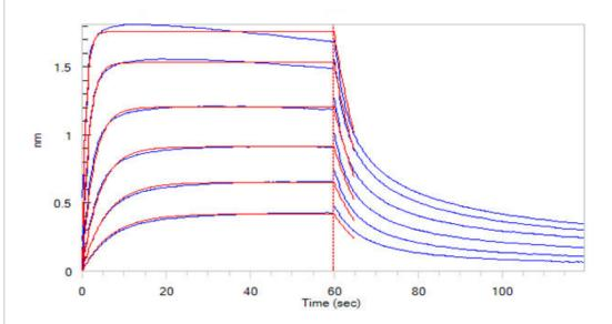
Loaded Rhesus macaque CD16, His Tag (Cat. No. FC6-R52H6) on HIS1K Biosensor, can bind Rituximab with an affinity constant of 0.28  $\mu$ M as determined in BLI assay (ForteBio Octet Red96e) (Routinely tested).
