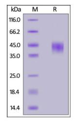
Biotinylated Mouse CD16, His, Avitag on SDS-PAGE under reducing (R) condition. The gel was stained overnight with Coomassie Blue. The purity of the protein is greater than 90%.
