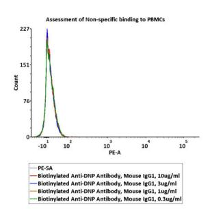
5e5 of PBMCs were stained with a series of concentrations of Biotinylated Mouse IgG1 Isotype Control (mAb) (Cat. No. DNP-BM1), washed and then followed by PE-SA and analyzed with FACS (QC tested).
