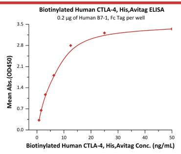
Immobilized Human B7-1, Fc Tag (Cat. No. <u>B71-H5259</u>) at 2  $\mu$ g/mL (100  $\mu$ L/well) can bind Biotinylated Human CTLA-4, His,Avitag (Cat. No. <u>CT4-H82E3</u>) with a linear range of 0.7-13 ng/mL (QC tested).
