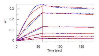
Loaded Human B7-1, Fc Tag (Cat. No. B71-H5259) on Protein A Biosensor, can bind Human CTLA-4, His Tag (Cat. No. CT4-H52H9) with an affinity constant of 0.498 nM as determined in BLI assay (ForteBio Octet Red96e) (Routinely tested).
