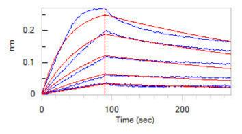
Loaded Human B7-2, Fc Tag (Cat. No. CD6-H5257) on Protein A Biosensor, can bind Human CTLA-4, His Tag (Cat. No. CT4-H52H9) with an affinity constant of 1.03 nM as determined in BLI assay (ForteBio Octet Red96e) (Routinely tested).
