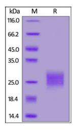
Human CTLA-4, His Tag on SDS-PAGE under reducing (R) condition. The gel was stained overnight with Coomassie Blue. The purity of the protein is greater than 90%.
