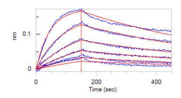
Loaded Cynomolgus CD3E&CD3D Heterodimer Protein, Fc,His Tag&Fc,Flag Tag (Cat. No. CDD-C52W9) on AHC Biosensor, can bind Bispecific CD3×BCMA T cell-engaging Antibody with an affinity constant of 1.77 nM as determined in BLI assay (ForteBio Octet Red96e) (Routinely tested).
