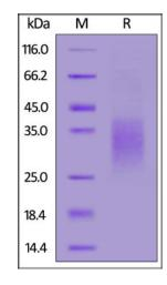
Human CD79A, His Tag on SDS-PAGE under reducing (R) condition. The gel was stained overnight with Coomassie Blue. The purity of the protein is greater than 90%.
