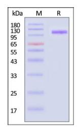
Mouse CD117, Fc Tag on SDS-PAGE under reducing (R) condition. The gel was stained with Coomassie Blue. The purity of the protein is greater than 95% (With Star Ribbon Pre-stained Protein Marker).
