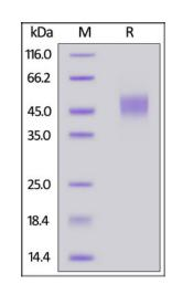
Biotinylated Mouse CD64, His, Avitag on SDS-PAGE under reducing (R) condition. The gel was stained overnight with Coomassie Blue. The purity of the protein is greater than 90%.
