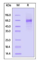
Biotinylated Cynomolgus B7-H7, His, Avitag on SDS-PAGE under reducing (R) condition. The gel was stained overnight with Coomassie Blue. The purity of the protein is greater than 90%.
