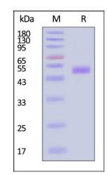
Human ANGPTL7 Protein, His Tag on SDS-PAGE under reducing (R) condition. The gel was stained with Coomassie Blue. The purity of the protein is greater than 90% (With <u>Star Ribbon Pre-stained Protein Marker</u>).
