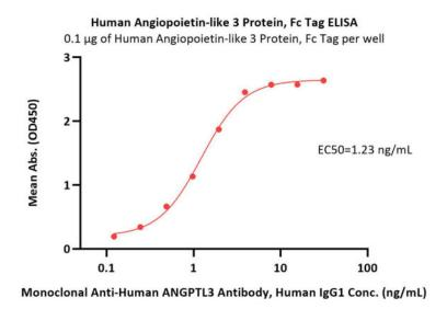
Immobilized Human Angiopoietin-like 3 Protein, Fc Tag (Cat. No. AN3-H5253) at 1  $\mu$ g/mL (100  $\mu$ L/well) can bind Monoclonal Anti-Human ANGPTL3 Antibody, Human IgG1 with a linear range of 0.1-2 ng/mL (QC tested).
