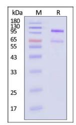
Human Angiopoietin-like 3 Protein, Fc Tag on SDS-PAGE under reducing (R) condition. The gel was stained with Coomassie Blue. The purity of the protein is greater than 90% (With <u>Star Ribbon Pre-stained Protein Marker</u>).
