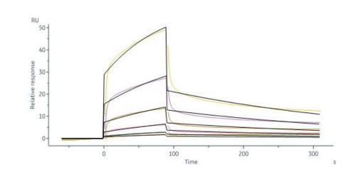
Rabbit Angiopoietin-2 Protein, His Tag (Cat. No. AN2-R52H4) captured on CM5 chip via anti-His antibody can bind Human TIE2, Fc Tag (Cat. No. TI2-H5255) with an affinity constant of 43.9 nM as determined in a SPR assay (Biacore 8K) (Routinely tested).
