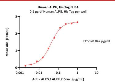
Immobilized Human ALPG, His Tag (Cat. No. ALG-H52H9) at 1  $\mu$ g/mL (100  $\mu$ L/well) can bind Anti - ALPG / ALPPL2 with a linear range of 0.002-0.125  $\mu$ g/mL (QC tested).
