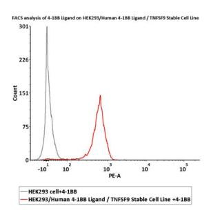
FACS assay shows that Biotinylated Human 4-1BB, Fc,Avitag (41B-H82F8) can bind to HEK293/Human 4-1BB Ligand / TNFSF9 Stable Cell Line (CHEK-ATP039). The concentration of Biotinylated Human 4-1BB, Fc,Avitag (41B-H82F8) used is 10 µg/mL (Routinely tested).
