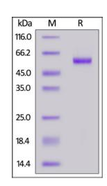
Biotinylated Human 4-1BB, Fc, Avitag on SDS-PAGE under reducing (R) condition. The gel was stained overnight with Coomassie Blue. The purity of the protein is greater than 95%.
