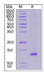
Human 4-1BB (24-86) Protein, His Tag on SDS-PAGE under reducing (R) condition. The gel was stained overnight with Coomassie Blue. The purity of the protein is greater than 90%.
